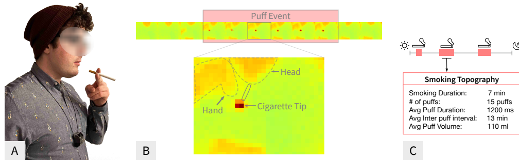
Fig. 1. SmokeMon is a chest-worn thermal-sensing wearable system with the lens pointed at the wearer [A] that can capture spatial, temporal, and thermal information around the wearer and cigarette [B] all-day to unobtrusively and passively detect smoking events and estimates of topography [C].
